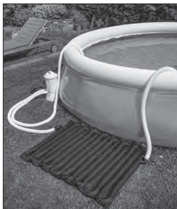
Solar Pool Water Heating
