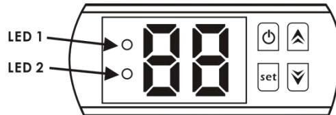
When the heat pump is running, the LED display shows the water inlet temperature.
