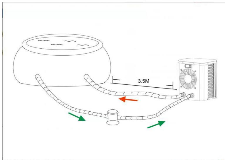
**ATTENTION:** Never install the unit in a closed room with a limited air volume in which the air expelled from the unit will be reused, or close to shrubbery that could block the air inlet. Such locations impair the continuous supply of fresh air, resulting in reduced efficiency and possibly preventing sufficient heat output.
